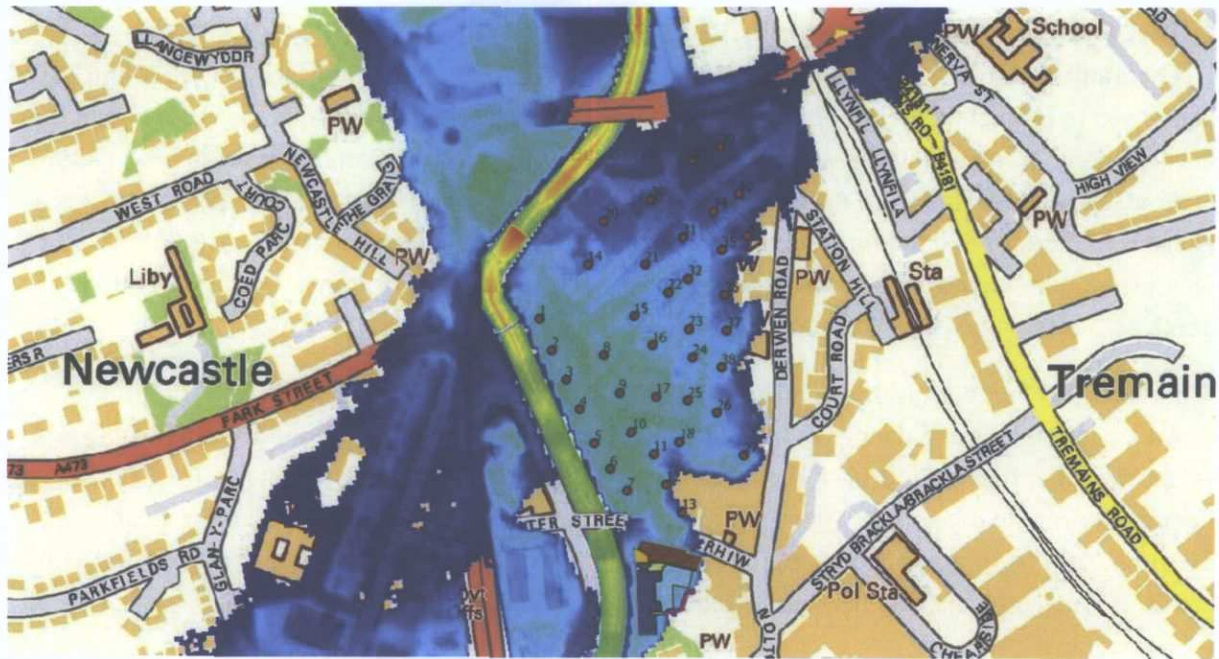
Figure 3 | Maximum water depths: 1 in 1000 year return period pre construction
