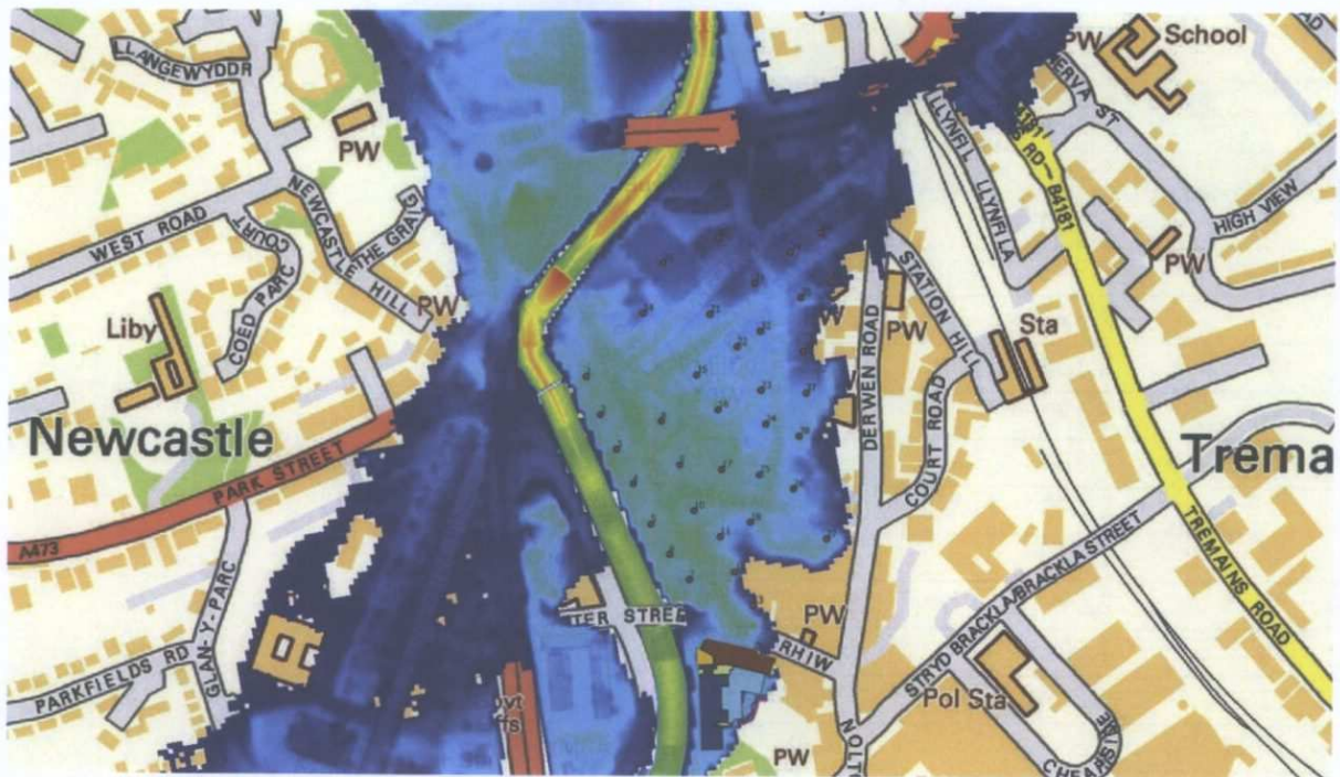
Figure 9 | Maximum water depths: 1 in 1000 year return period pre construction
