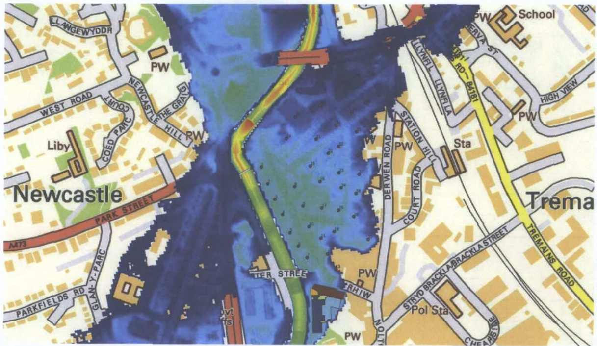
Figure 5 | Maximum water depths: 1 in 1000 year return period pre construction
